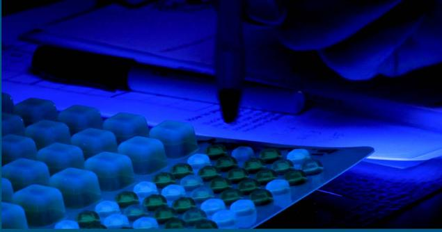
A lab technician checks water samples under UV light in the plant's lab. The Payson plant has consistently met the nondetectable effluent E. coli limit for ARIZONA TITLE 18 Class A+ reuse effluent.
