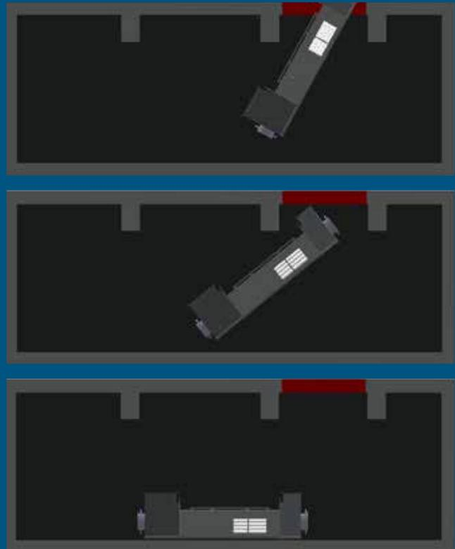
Fitting the new UV reactors through the access hatch at Sam Ludlow Sewer Plant
